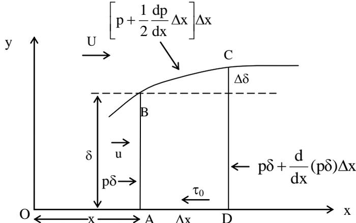
Let  $AD = \Delta x$  be the small length of the element in the  $x$ -direction and  $\delta$  be the thickness of the boundary layer at a distance  $x$  from the leading edge of the plate. We assume that the velocity of the boundary layer flow at the outer edge of the boundary layer is the same as that of the potential flow, i.e.,  $u = U$  at  $y = \delta$ .
