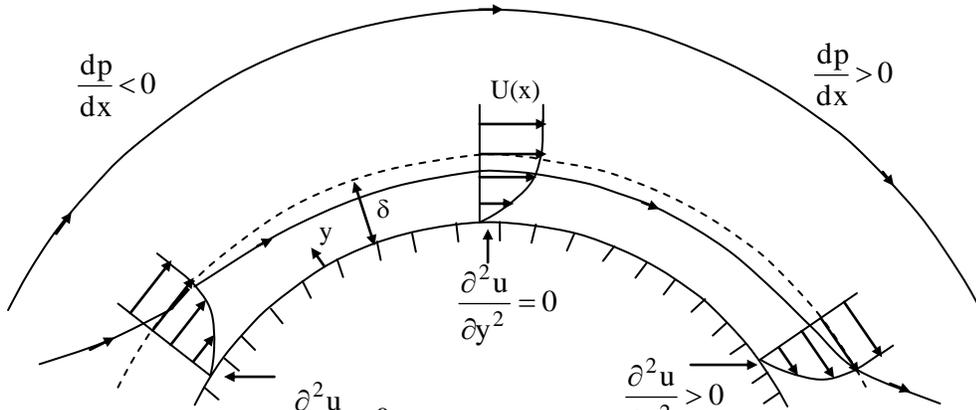
Upstream of the highest point the stream lines of the outer flow converge, resulting in an increase of the free stream velocity  $U(x)$  and a consequent fall of pressure with  $x$  ( $\frac{dp}{dx} < 0$ ) i.e. favourable pressure gradient. Downstream of the highest point the stream
